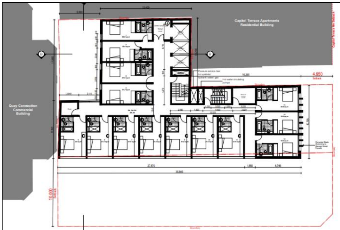
Figure 1 Approved Setbacks Above the Street Frontage (Levels 3 - 4)
